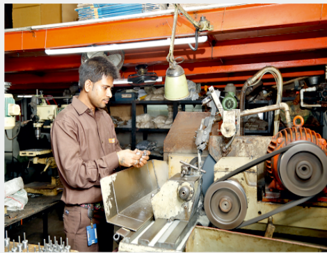
Cylindrical grinding process of rotors for 100% accuracy with tolerance achieved in microns.
